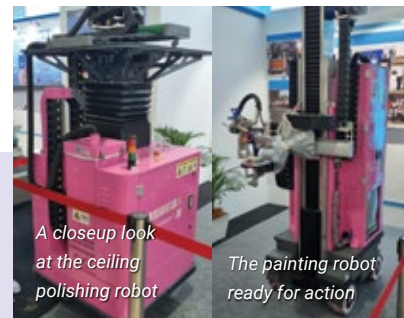
Hazardous and backbreaking ceiling polishing work being carried out by this robot
